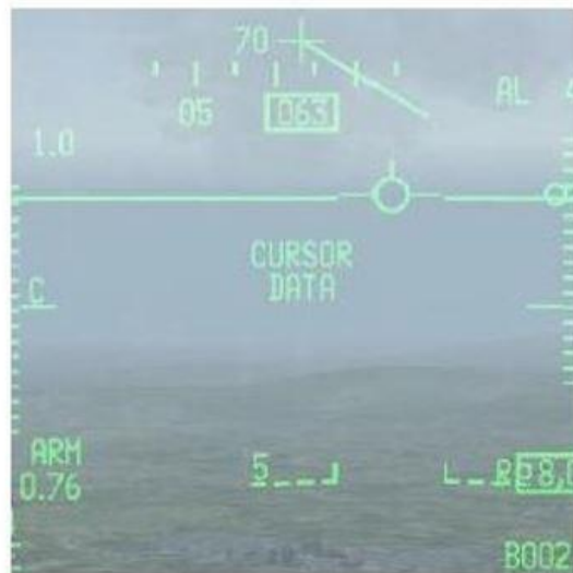
Figure 13 Assignee (#3's) FCR, HSD and HUD. Assigner (#1) sent cursor data NNE of ownship Markpoint
